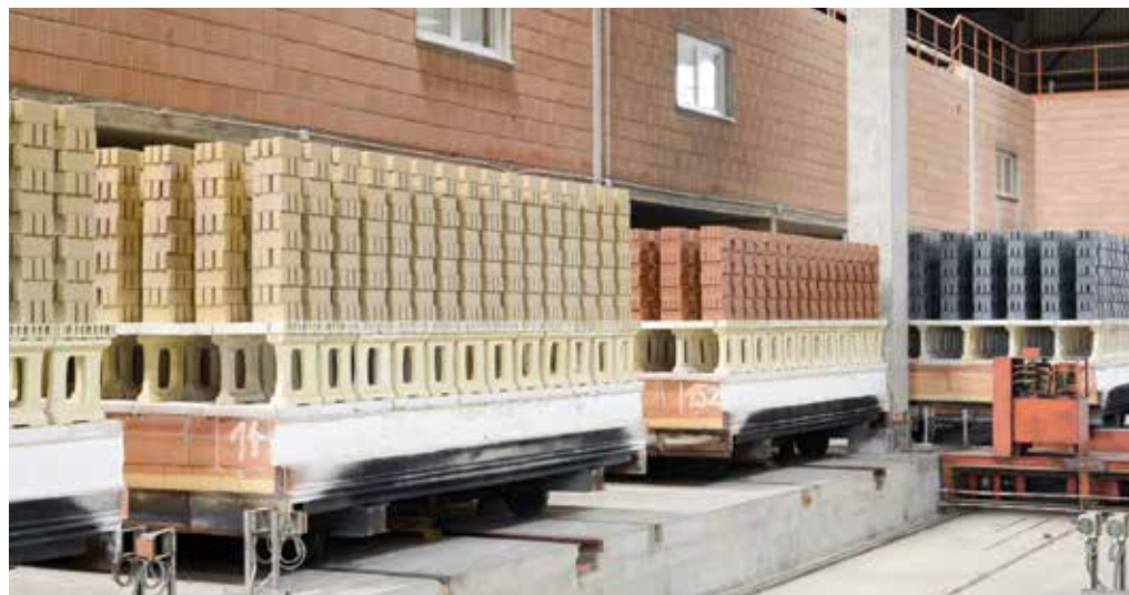
Tunnel kiln car setting with clinker pavers
