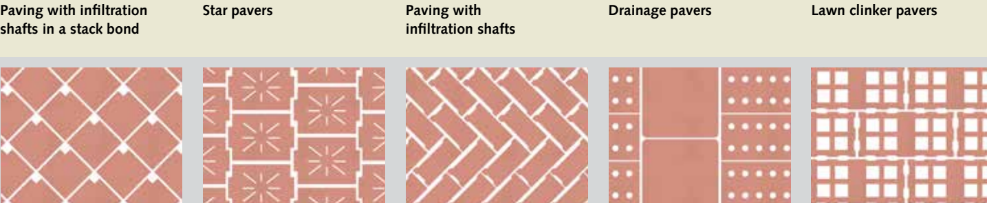
Fig. 6-3: Different clinker paver formats for permeable paving
