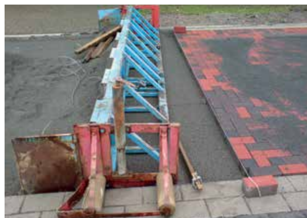
Fig. 5-10: Screeding of the bed surface using a screeding bar
