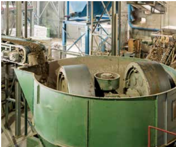
Pan mill, two heavy rollers comminute the clay
