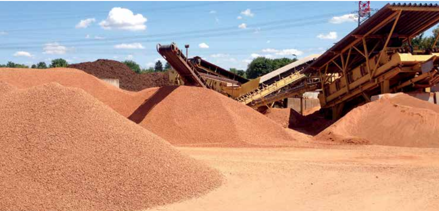
Production of recycled aggregates for use as substrate in vegetation engineering.
